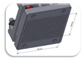
A presser of 195 x 145 mm for a total surface of 0,145 m is 0,028 m2
