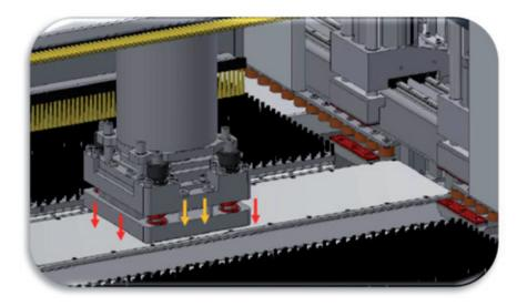
Presser operating pressure is 300/600 kg on the panel = 100 kg operating pressure on the panel
