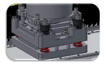
The mold of the Micra presser is interchangeable at any time according to the desired patterns.
