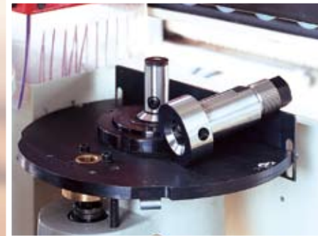
Manual quick tooling change system.
