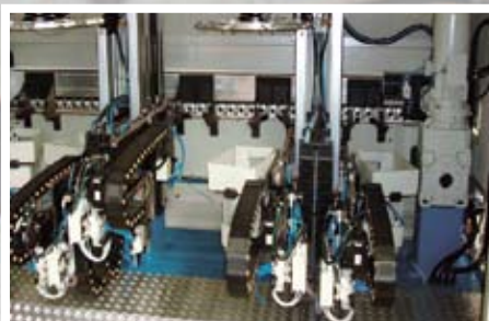
Machine equipped with carousel quick tool changing system.
